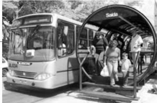
Brazil's BRT boarding islands provide for fare collection and a platform level with the bus, speeding both boarding and deboarding
