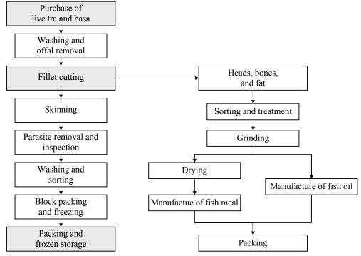
**Figure 1: Production Process of Frozen Fish Fillets**
